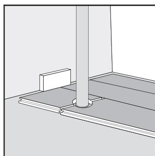
In rows where the flooring meets a pipe, ensure the pipe aligns exactly with the short sides of two panels.
