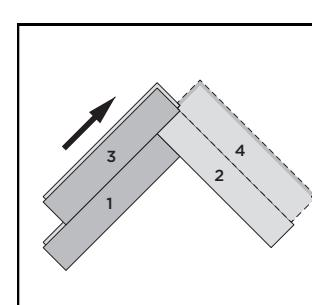
Angle up the long side of panel 3 into the long side of panel 2 at 20-30°, slide it towards panel 4 until it reaches the corner of panel 4 and angle down.
