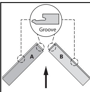
Lay down the panels in the correct start position with the groove side pointing away from the starter wall and to the outside of the V.
