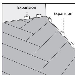
The floor must be able to expand and contract with changes in the indoor climate. For expansion joint guidelines, check the supplier's instructions.
