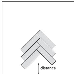
Start the installation at a distance away from the starter wall for easier installation.
