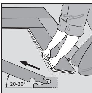
Start by angling out the panel by lifting the corner of the panel to about 20-30° and move the panel forwards and backwards until it releases.
