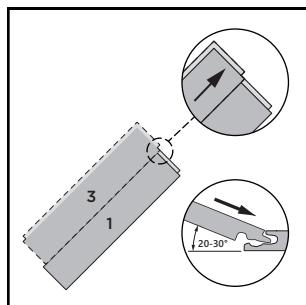
Use an alignment panel (3) to help align panel 2 by installing it 0,5 cm beyond the edge of panel 1.
