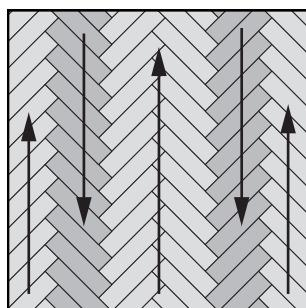
Complete the first V row with complete panels. Make sure to keep it aligned to the center line. Then continue on the sides, working in the opposite direction.
