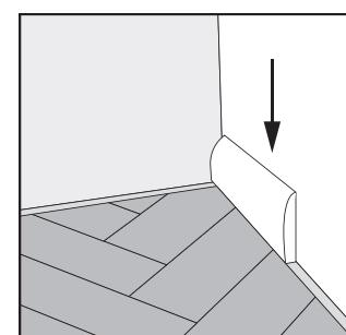
Install skirting on the walls over the expansion gaps to complete the room.
