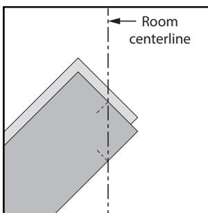
Align the markings on the panel to the center line of the room to ensure the correct angle of the panel and a straight installation.
