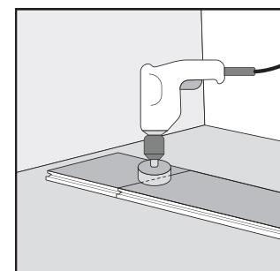
Click the panels together on the short side. Drill a hole centered on the joint between the two panels of the same diameter as the pipe plus 20 mm (3/4").
