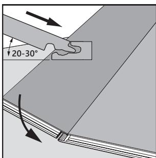
Start by locking in the long side. Position the panel at an angle of 20-30° to the panel that is already installed.
