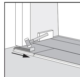
Slide the panel towards the already installed panels and gradually lock the short side of the panel with a tapping block or pull bar and hammer in a few taps.
