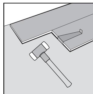
Place the pull bar against the panel. Gently tap the pull bar with a hammer to gradually connect the panels in a few taps.
