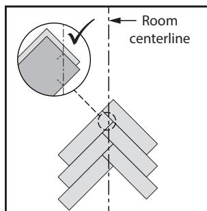
Align the rows to the middle line of the room, using the markings on the panel as a guide.
