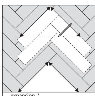
Mark the dimensions on the pre-build panels and cut to size. Install the remaining pieces one by one. Use a pull bar if necessary.
