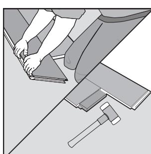
To install the next row, always connect the long side of the new panel into the installed panels. Use a tapping block to close the short side of the panel.
