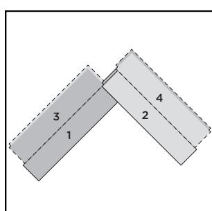
Use another alignment panel (4) to help align panel 3 by installing it 0,5 cm beyond the edge of panel 2.
