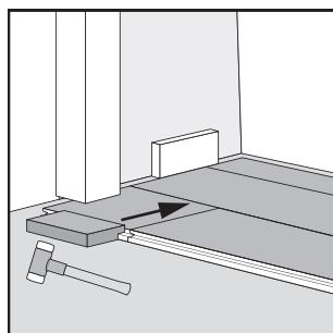
Install the panel on the long side with a tapping block or pull bar. Gently tap with a hammer to gradually connect the panels in a few taps.
