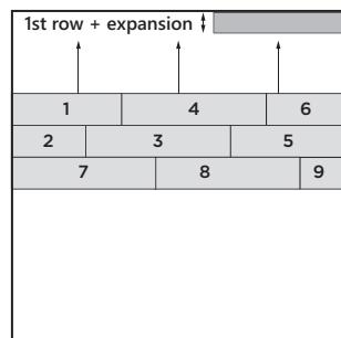
Move the rows closer to the wall, leaving a distance equal to the width of the start row plus the expansion gaps. Ensure the start row is at least 5 cm wide.
