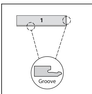
Start by positioning the first panel with the groove sides pointing away from the start walls.
