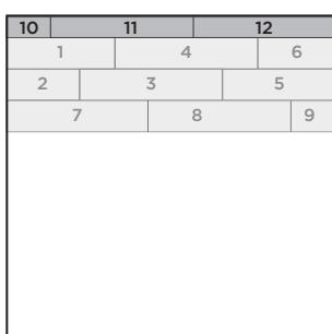
Install the start row by angling in the panels. Use the pull bar and hammer if necessary.
