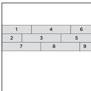
Continue installing the rest of the panels for the first three rows in the order of the drawing.
