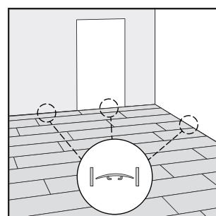
Provide expansion joints between different rooms or in large rooms. Check the supplier's guidelines for details.
