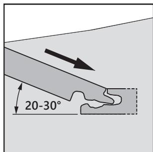
Place the tongue of the long side of panel 2 into the groove of the long side of panel 1 at 20-30° and angle down.
