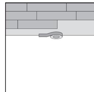
Lay the underlay parallel to the floor direction during installation. Start each new row of underlay upon reaching that point in the floor installation.
