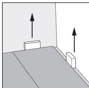
After the floor and expansion profiles are completely installed, remove all spacers from the room(s).
