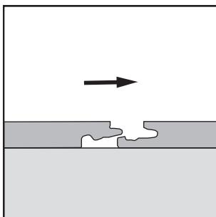
For hard to reach panels, use the tapping method. If possible, angle in one of the sides. Angle down and position the click systems as close as possible.
