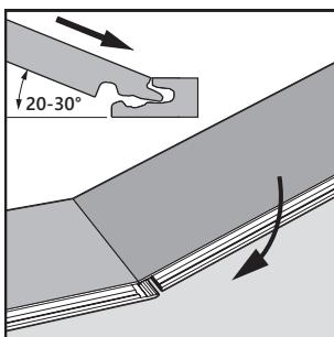
Start on the short side. Position the panel at an angle of 20-30° to the panel that is already installed, and angle down.
