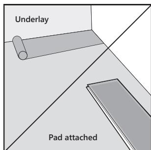
Check to see if there is a pad attached to the back of the panels.
